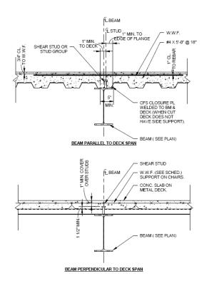
Figure 5: Typical Section Through Composite System
