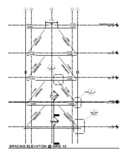
Figure 9: Eccentric Braced Frame
