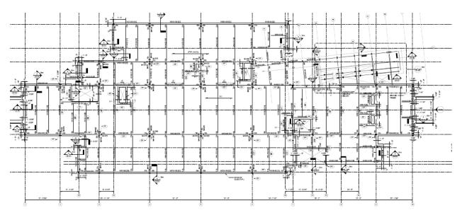
Figure 6: Typical Floor Framing Plan
