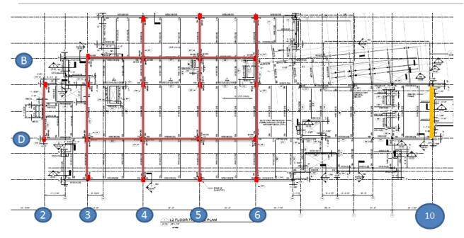
Figure 8: Location of Moment Connections (Red) and Braced Frame (Orange)
