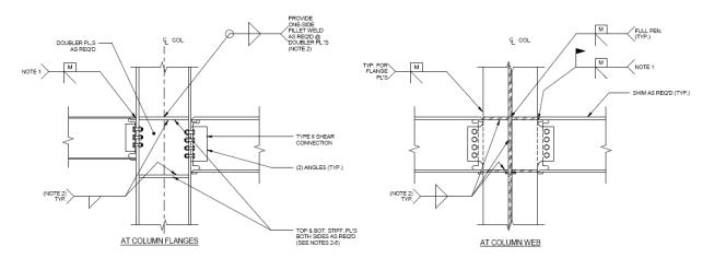
Figure 7: Typical Beam to Column Moment Connection
