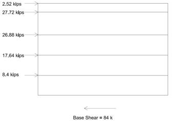
Figure 14: Vertical Distribution of seismic forces
